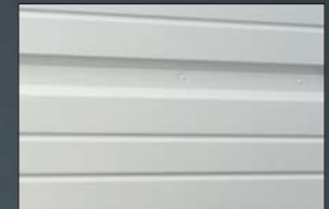
The face skin is attached to the box stiles using semi-tubular rivets vs. adhesives for added rigidity.
